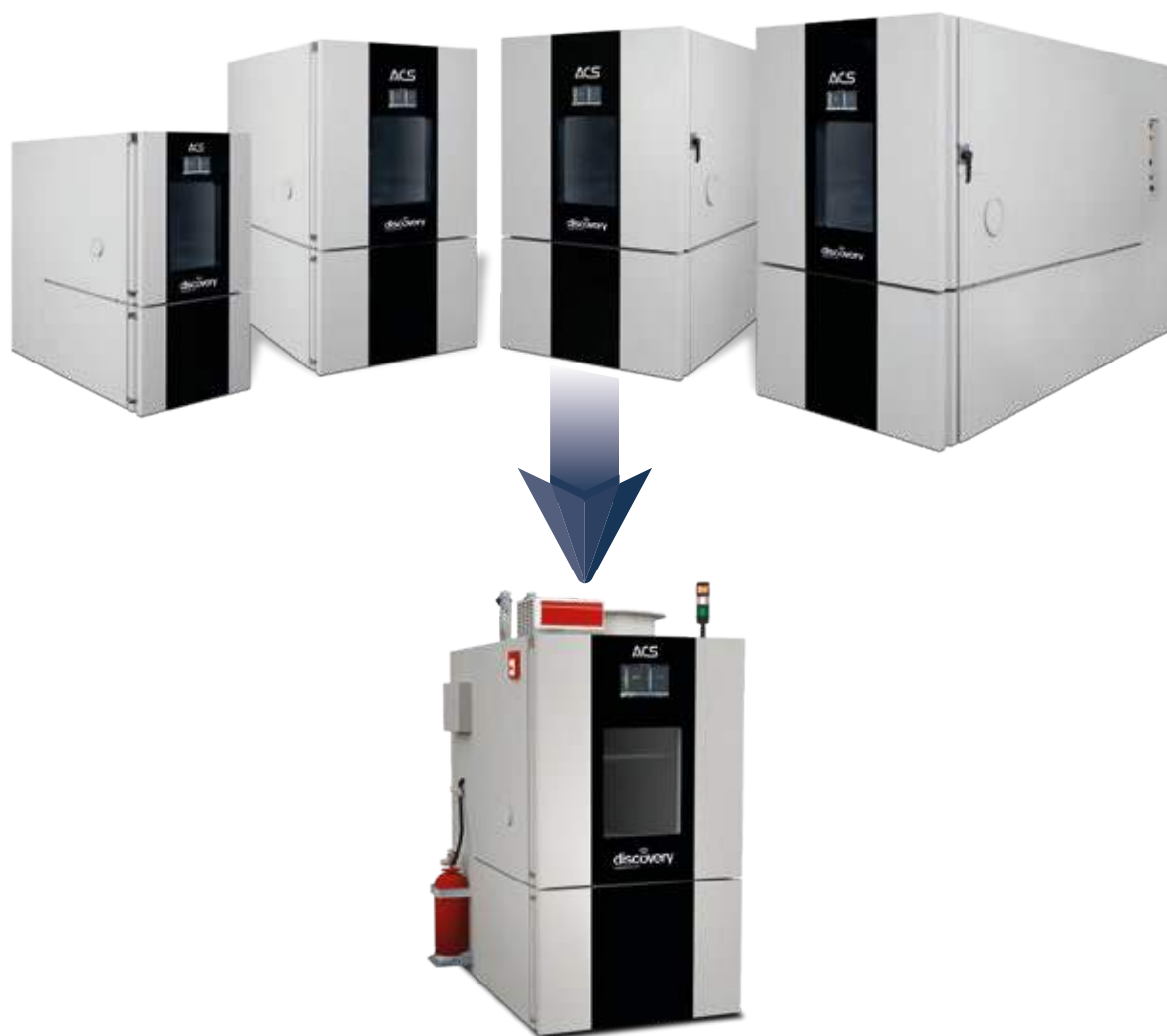
Sample of standard battery test solution
