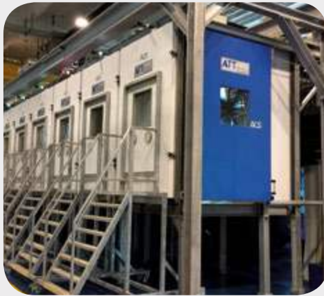
Walk in temperature, humidity and vibration test chamber (180 m 3 )
