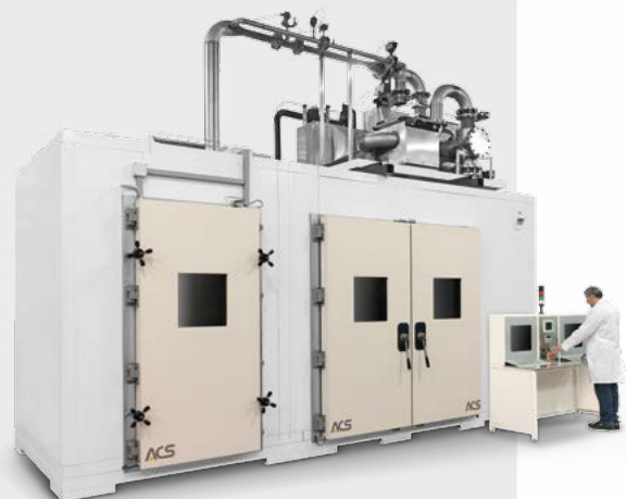
Calorimeter to measure the efficiency of air conditioning systems
